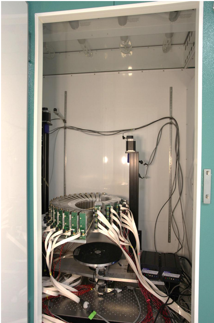
PET imager integrated in a plant growth chamber
