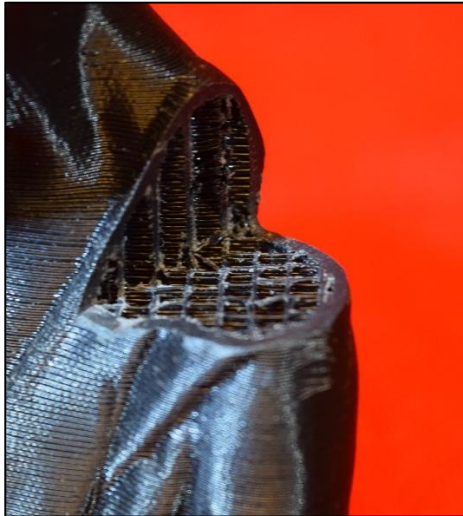
Figure 4: Sparse Low Density: Sparse Low Density uses the least amount of material and takes the least amount of time to print. It creates a grid-like pattern in the part that is mostly air. The outside several layers are still solid to help with part rigidity.
