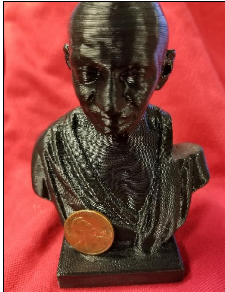
Figure 2: .010" Layer: This Layer height is the middle resolution and allows for a good-deal of features to show through and also prints faster than the .007" layer height. This is more cost effective than the .007" layer height option.
