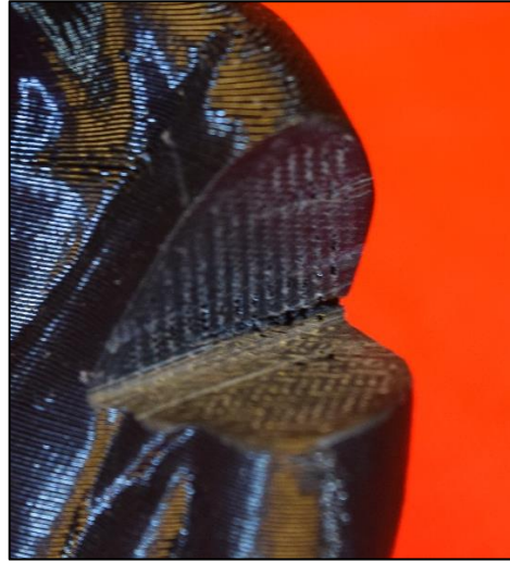
Figure 5: Sparse High Density: Sparse High Density uses the next amount of material and takes a "medium" amount of time to print. The internal pattern is a grid-like pattern that is almost equal parts air and material. The outside several layers are still solid to help with rigidity.
