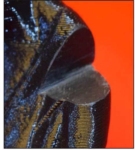
Figure 6: Solid: Solid internal structure takes the longest to print and uses the most amount of material. Since it is solid, the entire print is 100% print material. This will be the most durable and heaviest of all the print types.
