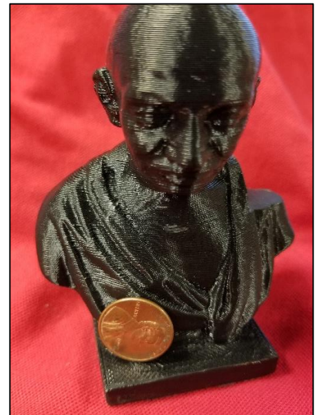
Figure 3: .013" Layer: This layer height is the courses height and misses the most of the part features. This is also significantly faster and most cost effective to print. The image shows that this resolution is still fairly good and will suffice for most prints.
