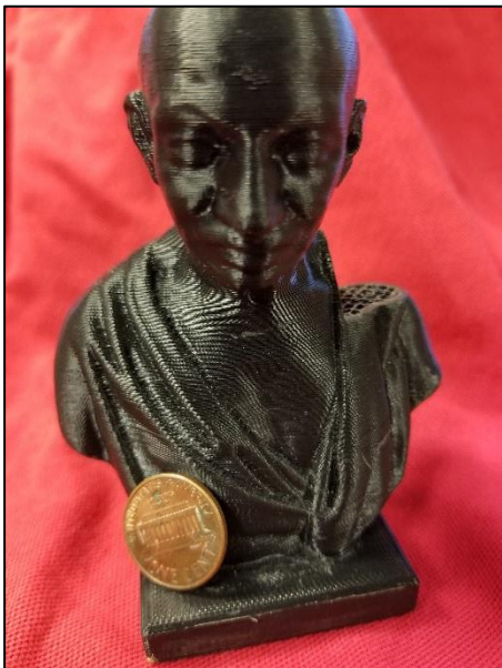
Figure 1: .007" Layer: .007" layer height allows for the best possible part resolution and will show most features. The print time for this height is very high and subsequently cost more than all the other layer heights.
