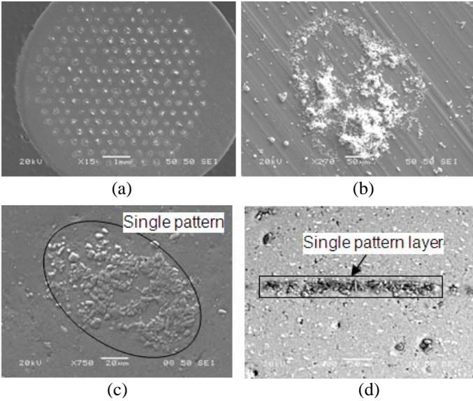
**Fig. 2** SEM images of spray deposition with pattern structures and consolidated composites.
