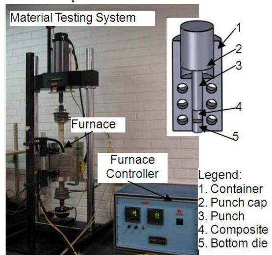
Fig. 1 Experimental setup for consolidation of composites.
