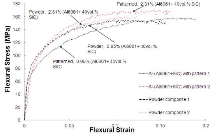
**Fig. 3** Flexural stress-strain curves of Al and composites.
